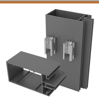
Universal die-cast aluminum bracket for sequential assembly of curtain wall systems. This double bracket can be used to install all transoms of the same series with different widths. This system eliminates the time-consuming installation by screws and allows a quick and accurate fastening thanks to the holes drilled on the mullion. With fixed anchoring buttons and safety screw. **Patented.**
