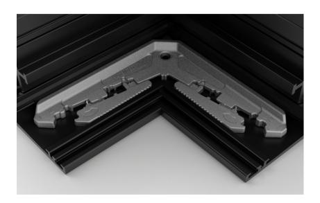
Die-cast aluminum corner joint with alignment and tightening function. Thanks to the two conical slides tightened with a simple slotted screwdriver, it aligns and closes the profile flawlessly. It can be installed on assembled profiles and, if necessary, easily disassembled. No profile processing is required. It has specific glue channels to guarantee perfect sealing and greater strength while avoiding any waste or spill. **Patented.**
