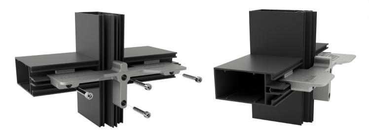
Die-cast aluminum support for heavy glazing of curtain walls. Adjustable depending on the glass thickness, assembled directly on the cross sections with self-drilling screws, avoiding the use of any additional frontal bracket. **Patented.**
